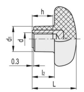
$\begin{array}{lll} D & = 32 \\ D1 & = 14 \\ DH & = M6 \\ h & = 10 \\ I2 & = 11.5 \\ L & = 23 \\ Weight in (g) = 19 \end{array}$
